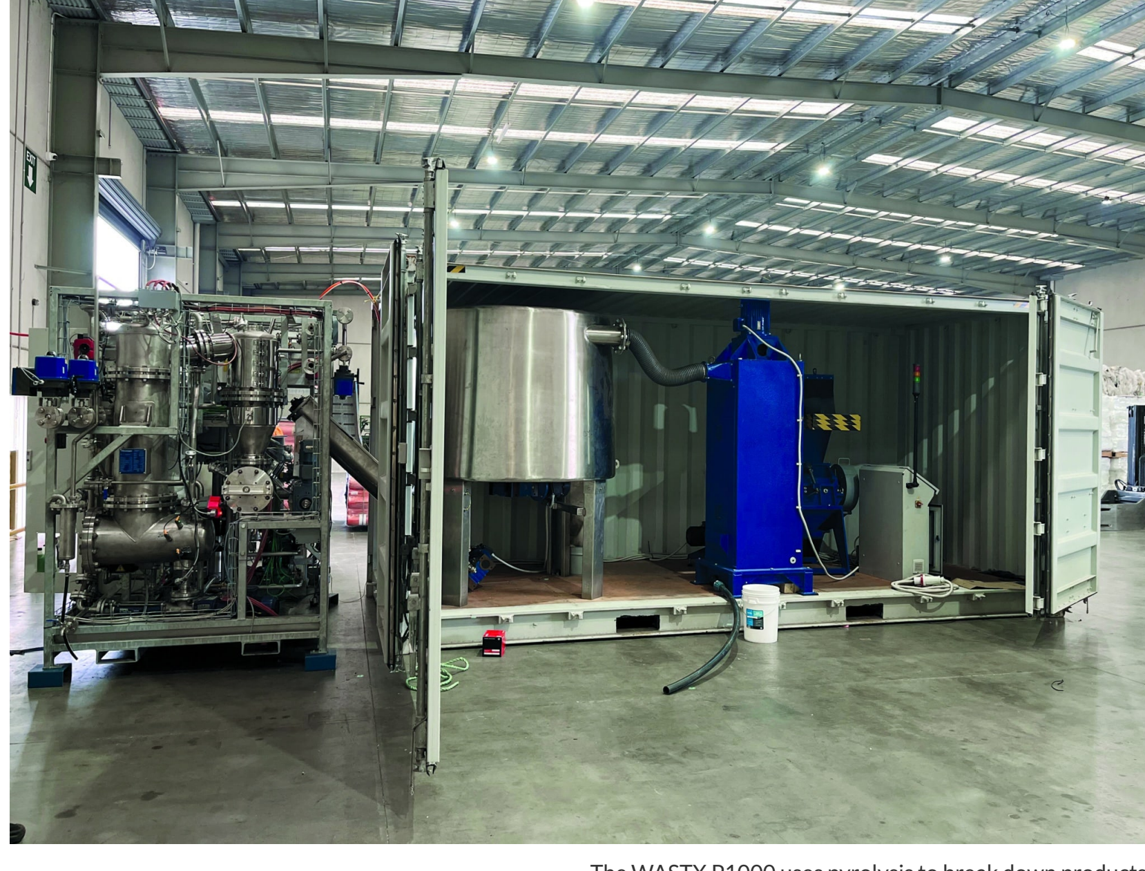
The WASTX P1000 uses pyrolysis to break down products.
